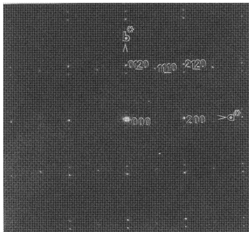
Fig. 1. The electron diffraction pattern with an incident beam along the [001] direction.
